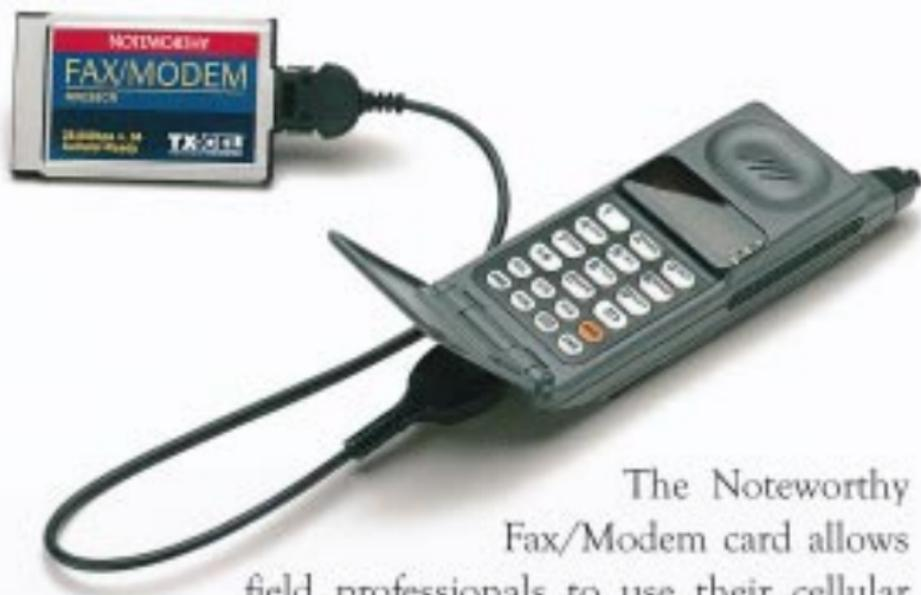
The Noteworthy Fax/Modem card allows field professionals to use their cellular phone to send and receive data and faxes. This Type II PC Card (PCMCIA) is cellular ready, providing 28.8kbps data transmission and 14.4kbps fax transmission.
